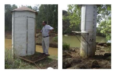
Picture showing Burial of automatic water level recorder (Abate et al. 2015) NB: GIS and remote sensing skill could have an added advantage
